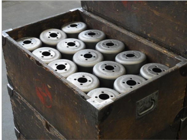
Picture 11: Bell knives are the core of each skiving machine.
