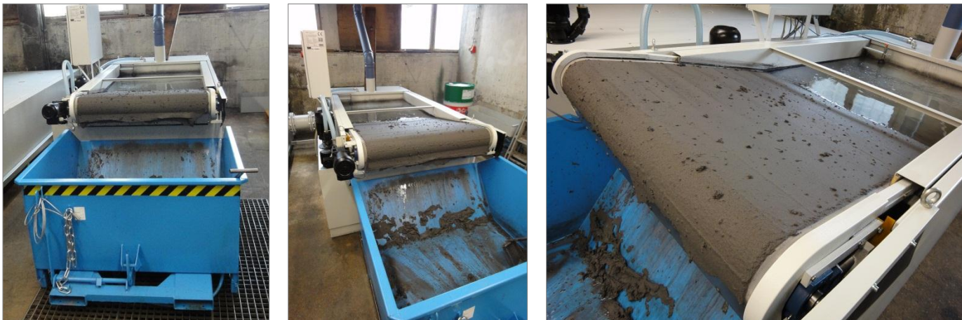
Picture 6–8: The MAXFLOW central system by GKD– Gebr. Kufferath AG. The self-cleaning stainless steel belt reliably protects against milling waste.
