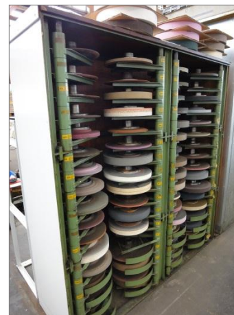
Picture 10: The production of high-precision single parts requires a number of different emery wheels.
