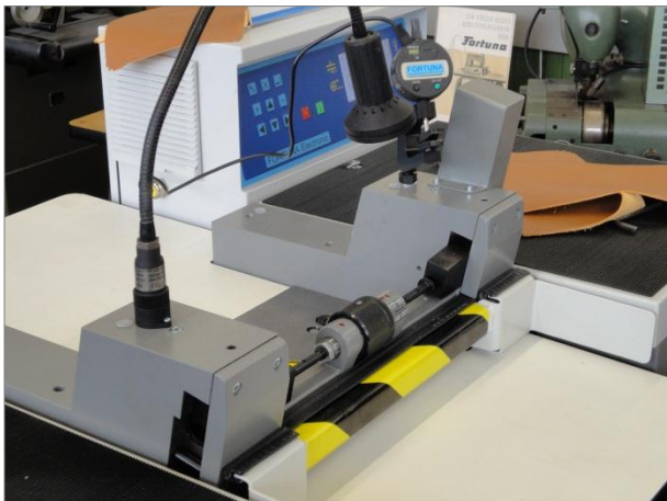
Picture 1–2: Precision bandknife splitting machines.
